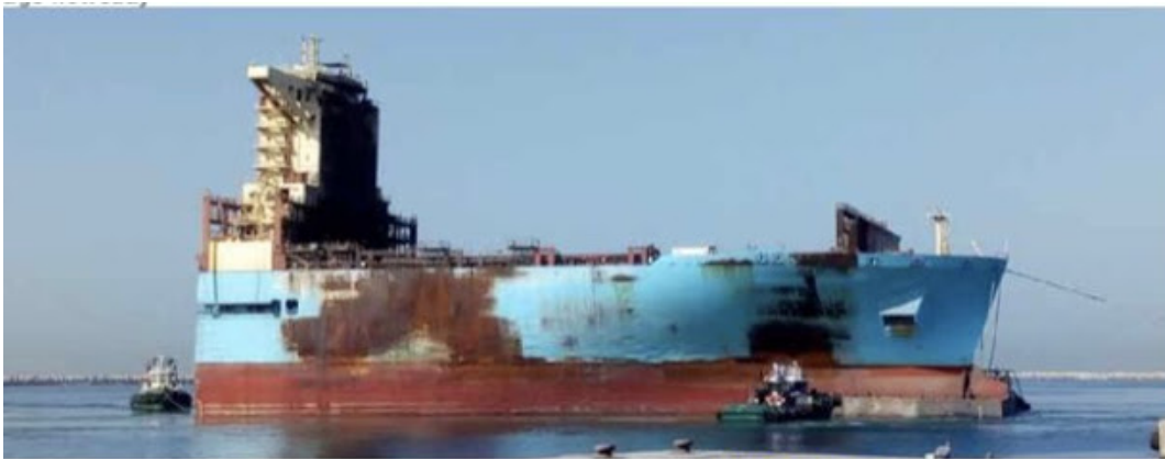
After have been cutted in two parts the forward section of the MAERSK HONAM shifting in Dubai
